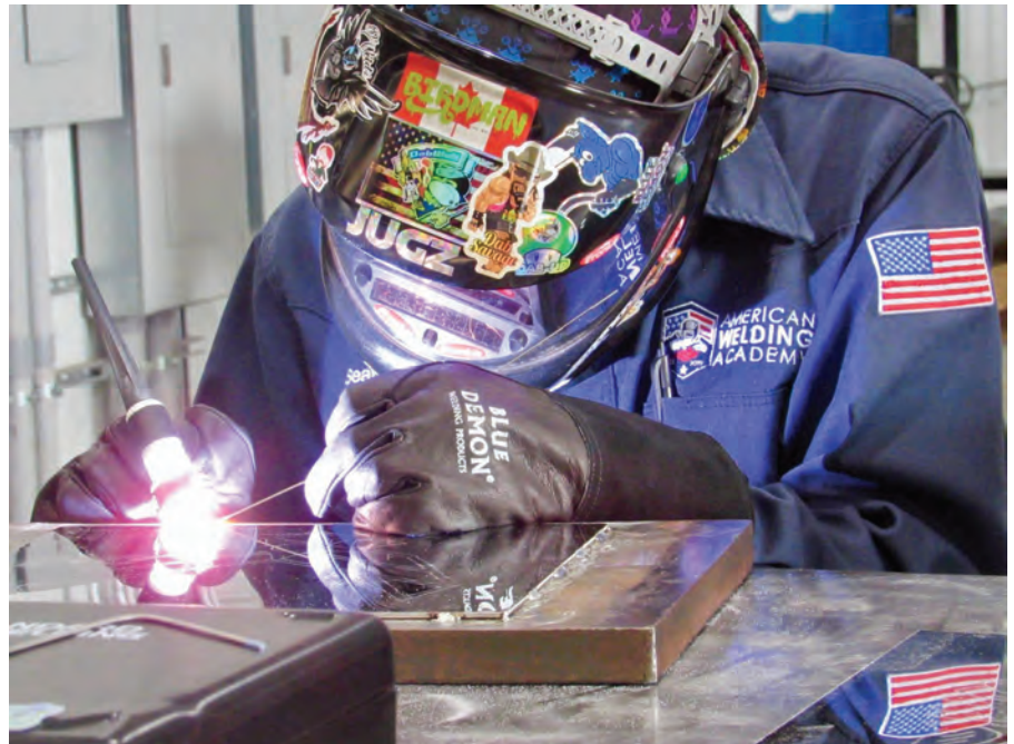
Fig. 4 — Sean “Dabs” Flottmann demonstrates his gas tungsten arc welding artwork on mirror polished stainless steel.
