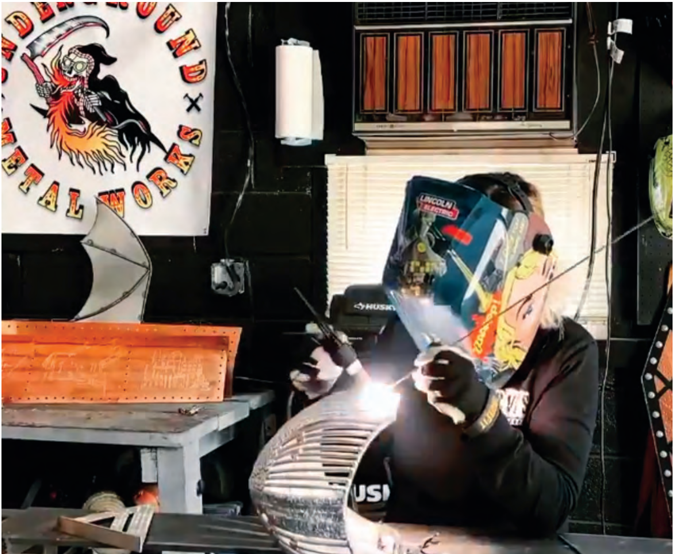
Fig. 2 — Hoffman uses a welding back filling technique to fill in gaps on the aluminum helmet. Credit: Stephanie Hoffman (@underground_metal_works)/Instagram.
