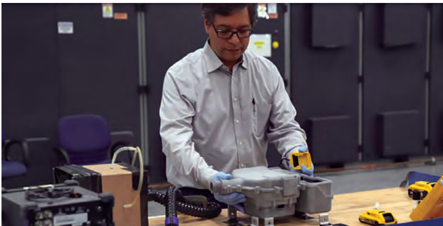
Fig. 4 — An engineer assembles the battery system for the new PAPR using two types of DeWalt batteries. (Photo credit: Ford.)
