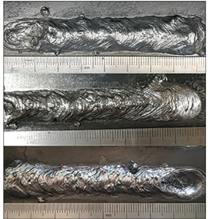
Fig. 12 — Comparison of weld bead appearance under the original waveform (left) and the optimized waveform (right).
